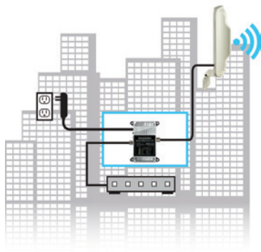
Typical Installation Stealth M2M X6 (Fig. 3)
