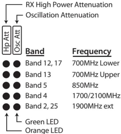
The “LEDS” on the face of the booster indicate operating gain state. In any given frequency band.
